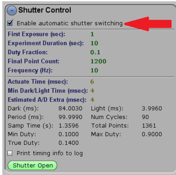
This mode will allow for an initial exposure of your sample, then subsequent exposures based on a user defined "Duty Fraction".
