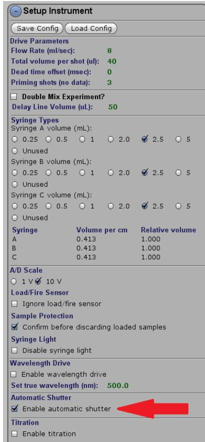
After restarting the software, this will activate the “Shutter Control” section of the software. Simply enabling the automatic shutter will automate shutter control for tasks such as dark current and reference readings.
