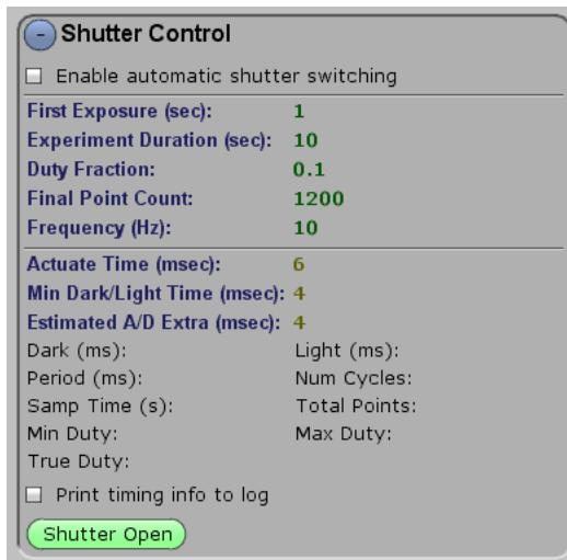
Enabling automatic shutter switching will activate the shutter during data collection mode.
