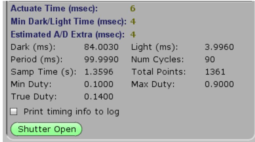
1. **Actuate Time (msec):** This defines the amount of time it takes for the electromechanical system to open a shutter or turn on a light source (LED). This value may be slightly different for each shutter or LED.
