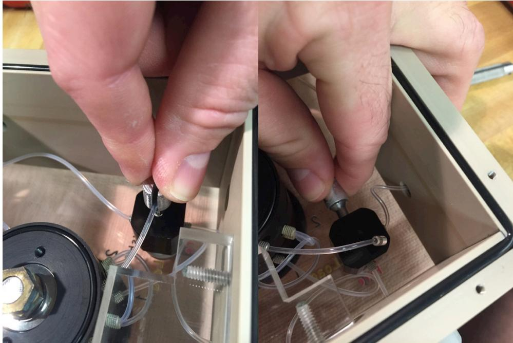
**The flush line should remain in the valve.**
