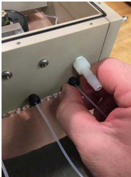
7. Flip the syringe box over and first remove the valve handle using the supplied 0.050" allen key. Then remove the nut that secures the valve with a 1/2" wrench.
