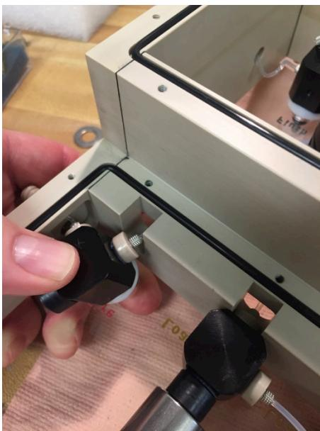
**11. Use microtubing wrench to remove load loop from the minstac valve adapter.**
