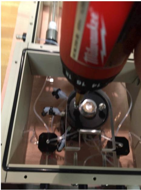
**5. Use microtubing connector wrench to remove the Sample load loop form the back of the lower valve and the valve to valve buffer line from the top of the valve.**
