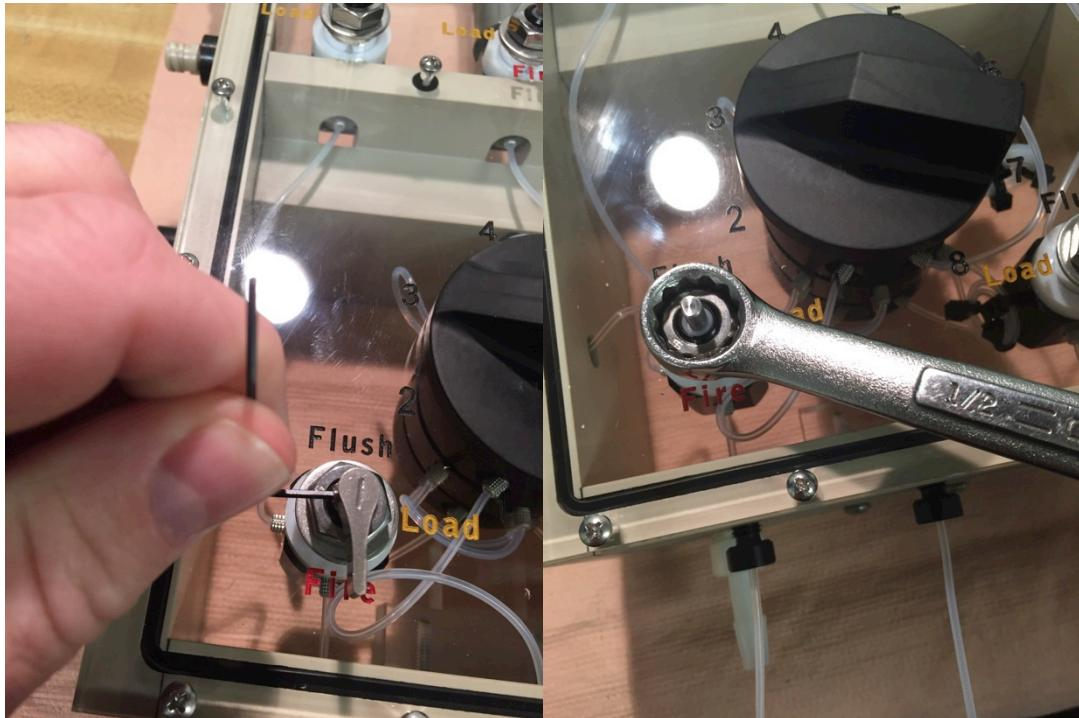
If removing the lower valve it is now free and can be removed from the syringe box. Carefully feed the flush line out of the bottom of the box. Flush line will be reused in new valve as will the white Teflon spacer on the stem of the valve.
