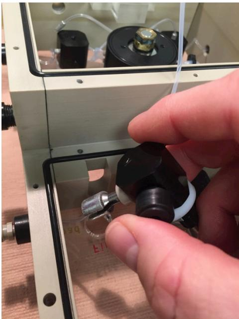
**12. Upper valve removed from the syringe box. Note that all fittings are in place as is the valve-to-valve buffer line. The plastic fittings (2x minstac adapters, syringe adapter and Teflon spacer) will all be reused on the replacement valve.**
