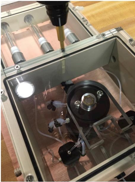
**4. Remove the acrylic “Tombstone” from the back of the 8-way valve to give additional work space.**
