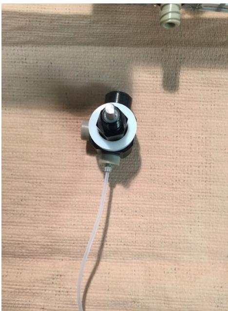
**13. Reinstallation is reverse of removal. Thread sealant or Teflon tape may be used on the plastic fittings to ensure a leak free seal but nothing should be used on the minstac fittings. Do not over tighten and of the fittings into the valves as this can lead to premature valve failure. Once you feel the fitting bottom out in the bore turn an additional  $\frac{1}{4}$  turn to ensure a good seal.**
