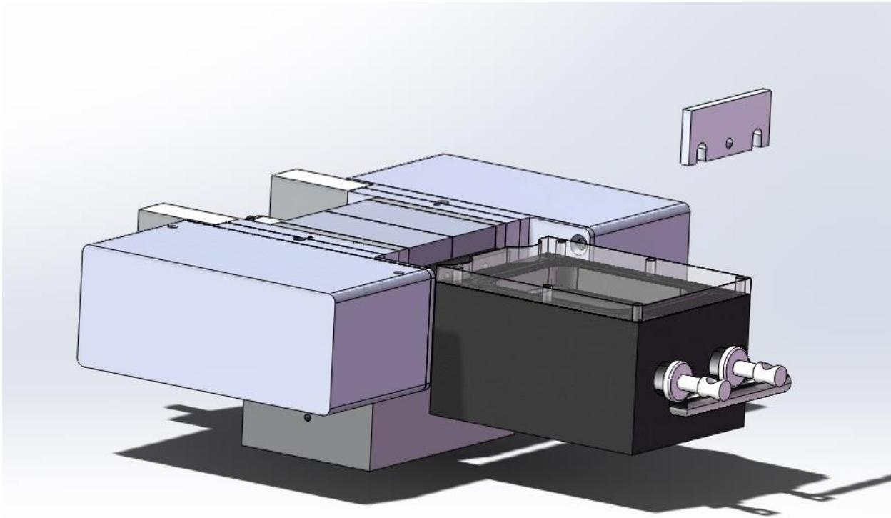
Using a 3/32 hex driver, remove the syringe retainer from the assembly by removing the screw and lifting up. When replacing this screw, ensure NOT to tighten it. The screw simply should make contact with the retainer so that it stays in place. Tightening this screw will put undue lateral pressure on the syringes and they may break.
