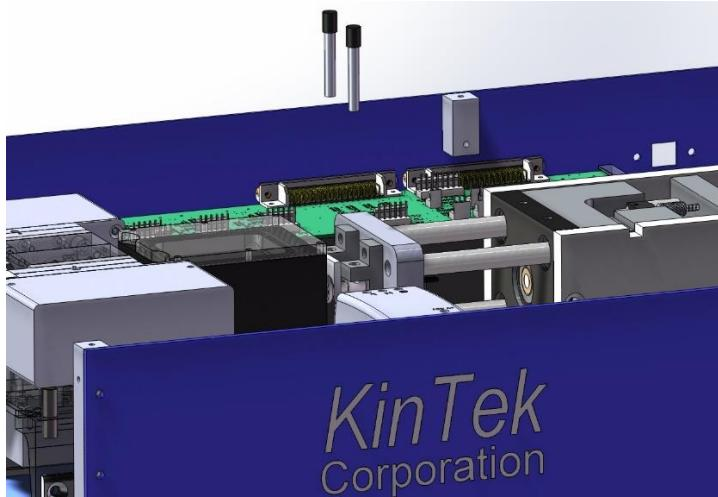
Remove the syringe plunger pins from the drive plate brackets. These two pins should simply pull out.
