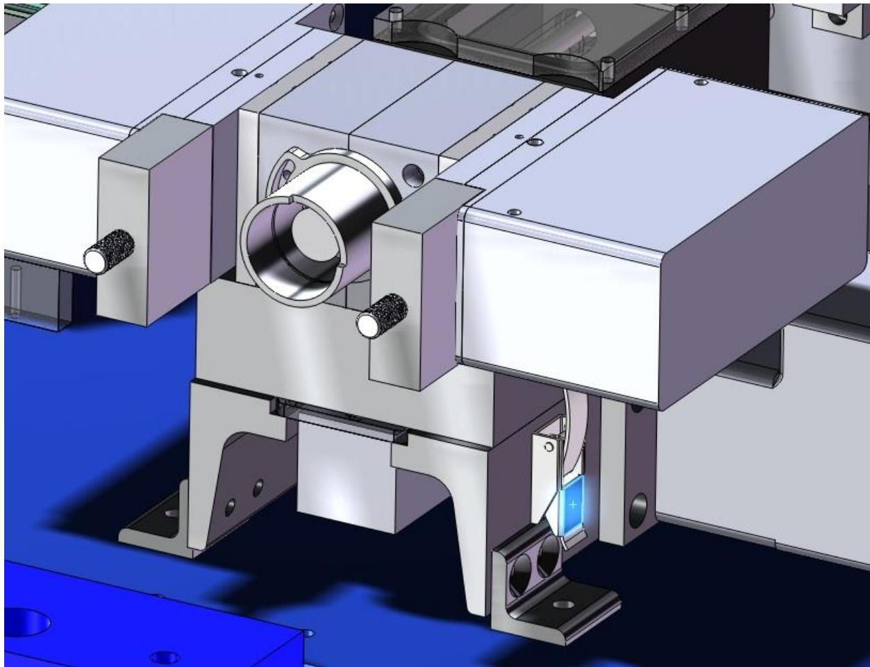
There are two spring-loaded clips holding the syringe assembly in place. They are located under the PMT modules as shown (one on each side). Lift out and up on these clips to release them.
