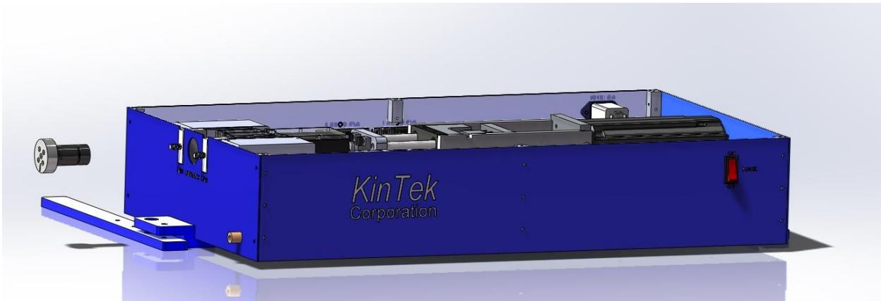
Remove the round fiber adapter from the left side plate. This fiber adapter simply pulls out (with some effort). It is held in place by an o-ring.
