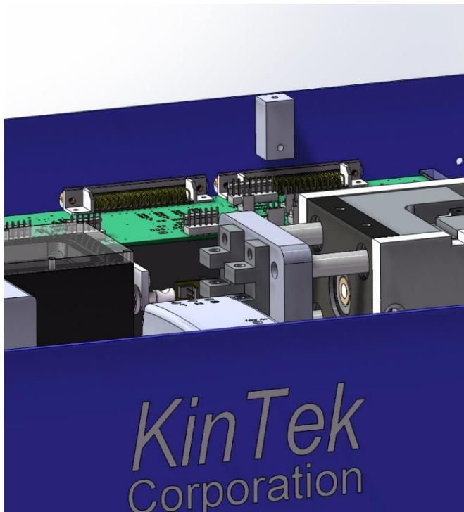
Move the drive plate to the right so that the plungers clear the drive plate brackets when the syringe assembly is lifted out. Ensure the water bath tubes are disconnected, the LED power wire is disconnected and the temperature probe is removed. When disconnecting water lines and removing the temperature probe, be aware that if the system isn't drained, water will escape from the chamber.
