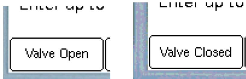
If the stop valve is opened manually, and left open, it automatically closes after 5 minutes.
